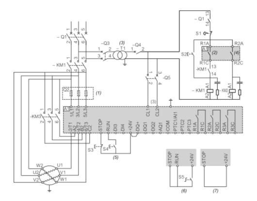
Connection inside the delta, with line and bypass contactor, type 1 and 2 coordination, non reversing, 2 wire or 3 wire
